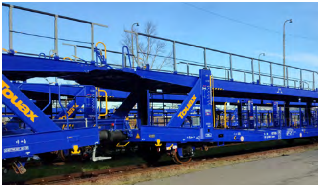
New Laaers car-carrier wagons
